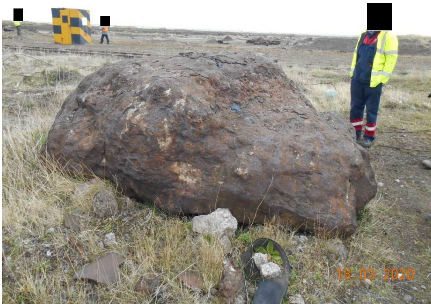
Plate 9 - Typical example of waste iron blocks discarded across land south of the torpedo pond area. Estimated size 5.0 X 5.0 X 1.5m.
